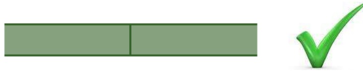
Fig 2c. Cavity barrier correctly fixed with no gaps
